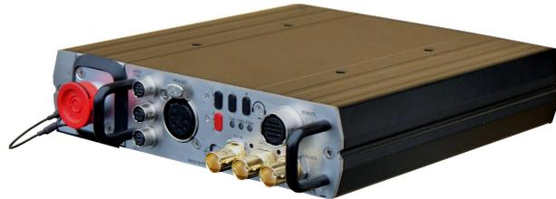
The Camiflex product has been developed to simplify the deployment of cameras for PTZ, OB Van, Studio and Cinema applications: the numerous cables between the camera and the control room are now over, a simple optical fiber to deploy and you're ready to go.
